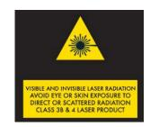
**OPTICAL HAZARD:** Laser operators should be aware of the potential hazards of Lasers, such as optical injury caused by unintended irradiation of the eye. Hazard reduction, such as the provision of appropriate safety eyewear, removal or covering of reflective surfaces in the treatment area, and adequate signage and removal of the key when not in use is the responsibility of the Laser user.
